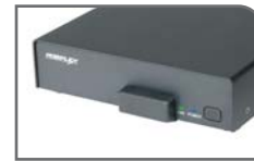
CF card slot with security cover for thin-client network architecture application.(CF card optional)
